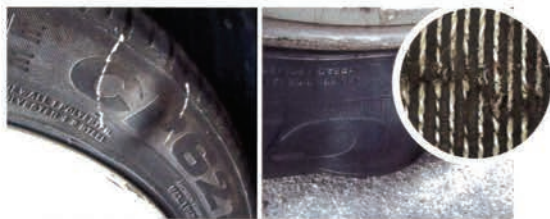
Localized protrusion in the sidewall
